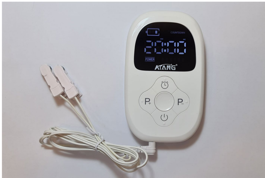
Fig. 1 ATANG CES (AT-9 model), including the main body, wires, and the electrodes which are connected to the patients' earlobes
